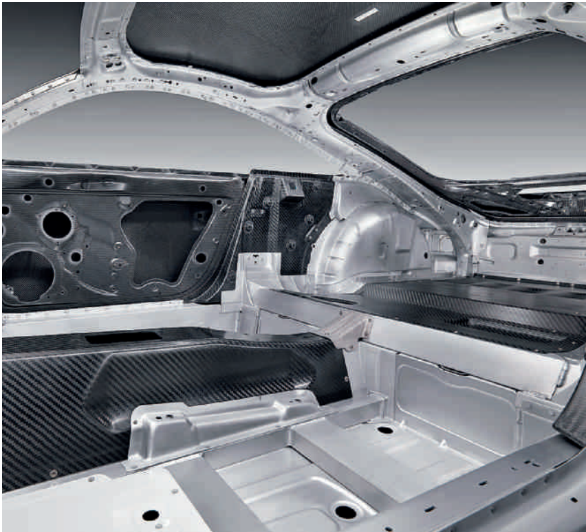
Perfectly combined: The newest joining technologies are used in the multimaterial body of the Audi TT ultra concept.
